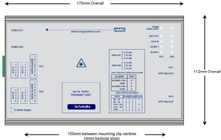
The **AMG5515A1B1** is a standalone transmit unit designed to transmit two Uni-directional alarms, and transmit & receive 3 data signals Bi-directional data signals over a Singlemode optical fibre.
